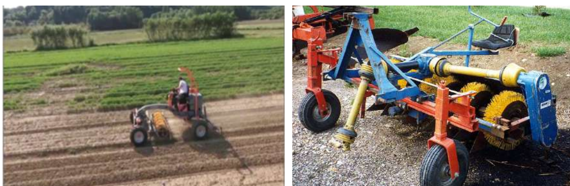
Figure 24. The horizontal axis brush hoe (left: mounted on a specialised tool-carrier tractor)
