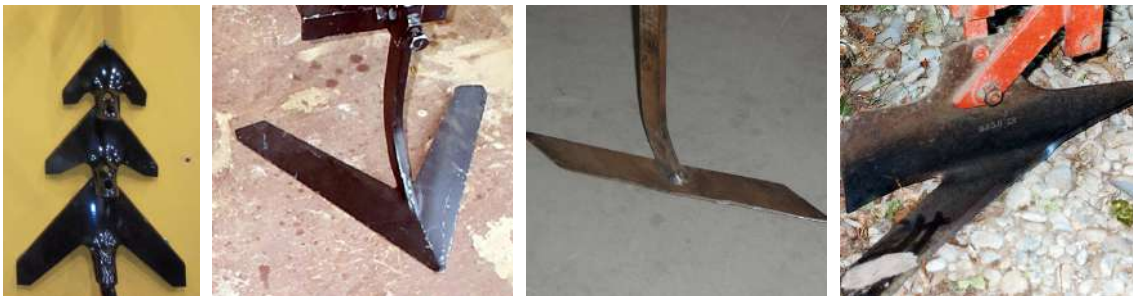
Figure 21. Interrow hoe blade designs, left to right: duck or goose foot, A blade sweep, L blade hoe, T hoe
