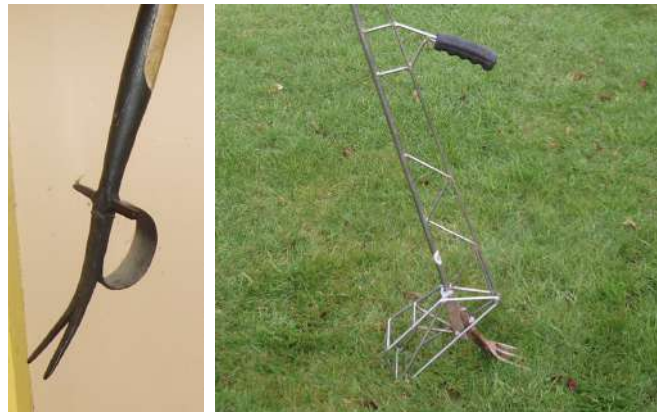
Figure 5. Traditional dock fork (left), modern ergonomic design with interchangeable heads (right) ( LazyDogTools.co.uk )
